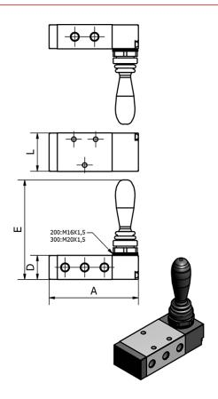
$\begin{array}{lll} A & = 101 \\ D & = 27 \\ E & = 93.5 \\ L & = 40 \\ Port & = G3/8" \\ Port \ exit & = G1/4" \\ Port \ supply \ and \ blowdown = G3/8" \end{array}$
